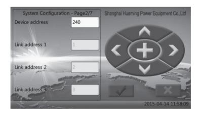
Device address: Set up SHM-K communication protocol's device address, the default value is OK.
