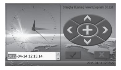
System time setup, select the year, month, day ,hour, minute, second by press left, right button, and upper and lower buttons to increase or decrease. The setup of timing can help the user to know the working record of the motor drive unit from the history log.
