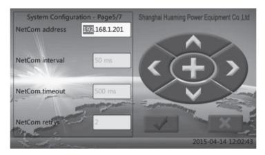
When the way of linking is network synchronization, then this screen is to set up the destination SHM-K's network address and its communication parameters. When the way of linking is optical, the parameter is not meaningful. The destination SHM-K must open the network expansion function and the protocol must be Huaming user defined.
