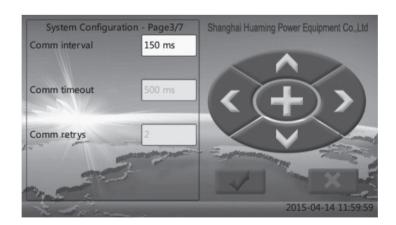
Communication interval: it shows the shortest time difference between the two communications
