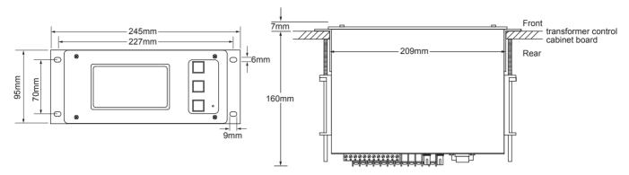
Installation can be done by the screws in front panel, also can be adopted as upper right side of the bayonet lock installation.
