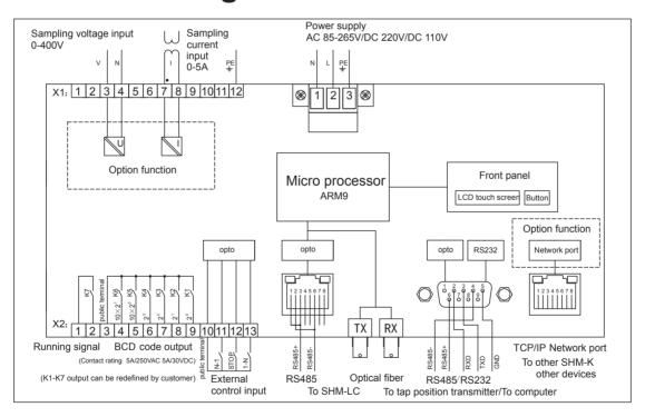
• Power Supply AC 85 ~ 265V or DC 110V, 220V input
