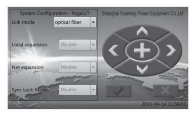
**The way of linking:** It is used to obtain real-time data from the MDU. The default mode is by optical fiber. A total of four modes can be selected: optical fiber, optical fiber mode 2, the fiber mode 3, the network synchronization.
