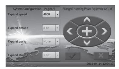
When turn on the local expansion function, it is used for setting up the CDT protocol communication parameters. If the local expansion not opened, the parameter is not meaningful.
