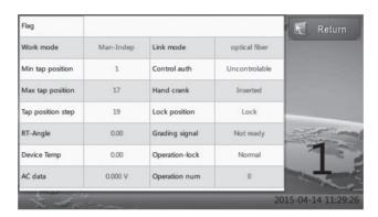
On the screen lower right corner it shows the current tap position, click the "return" button on the upper right corner can return to the main interface.
