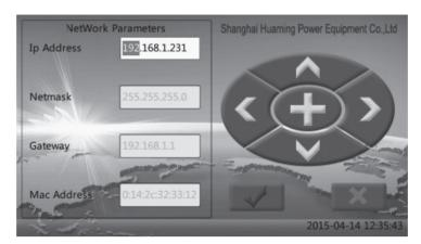
When the SHM-K working under parallel mode or under network synchronization need to set up network address or related parameters, the network address must be routable
