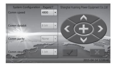
Set up the optical fiber communication parameters, normally use default value is OK.
