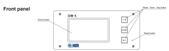
Reset button can be used for remote controller restart
