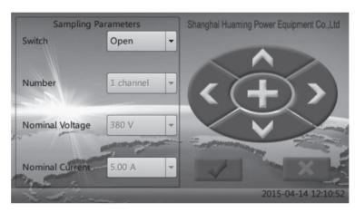
When the system is operating in auto voltage regulation mode, the screen is used to set the parameters in compliance with AC-tuning to ensure the accuracy of the data.
